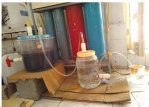
Fig 1 showing the experimental setup i.e. anaerobic digester
