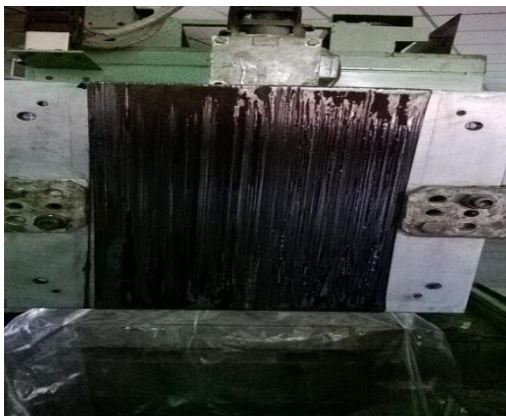
Fig.1 Carbon roving/Epoxy UD laminate winding by Filament Winding
