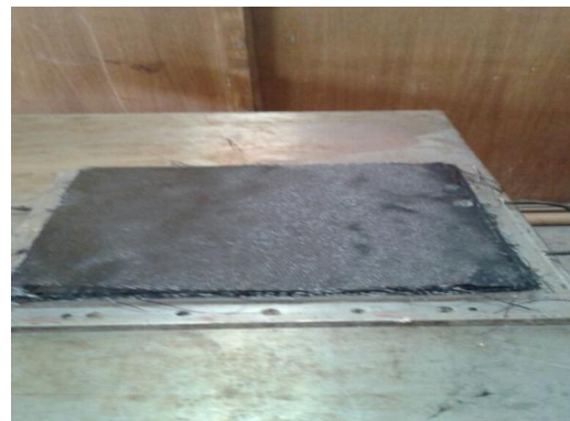
Fig.2 Carbon fabric/Epoxy BD laminate by Hand-layup
