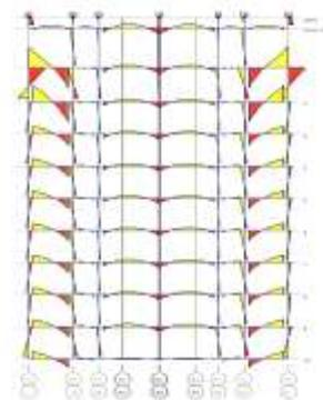
(h) case 4 (Removal of critical columns C-31, C-12, C-76 in y direction)
