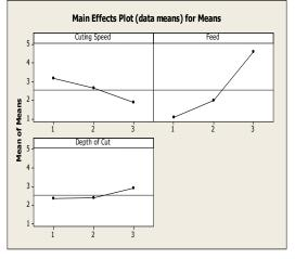
From Table 5, it is clear that feed is the most influencing factor followed by cutting speed and depth of cut for surface roughness. The optimum value for surface roughness is predicted from Fig 2, i.e. cutting speed of 938 rpm, feed of 0.0625 mm/rev and depth of cut of 0.2 mm.
