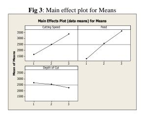
From Table 6, it is clear that feed is the most influencing factor followed by cutting speed and depth of cut for MRR. The optimum value for MRR is predicted from fig 3, i.e. cutting speed of 938 rpm, feed of 0.1875 mm/rev and depth of cut of 0.2 mm.
