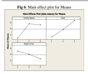
From Table 9, it is clear that feed is the most influencing factor followed by cutting speed and depth of cut for surface roughness. The optimum value for surface roughness is predicted from Fig 6, i.e. cutting speed of 384 rpm, feed of 0.0625 mm/rev and depth of cut of 0.4 mm.From Fig 9 and 10 it is clear that the HSS tool is the most suitable tool for minimized surface roughness and maximized material removal rate with maximum speed when compared to Carbide and PCD tools.
