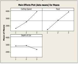
From Table 8, it is clear that feed is the most influencing factor followed by cutting speed and depth of cut for MRR. The optimum value for MRR is predicted from Fig 5, i.e. cutting speed of 938 rpm, feed of 0.1875 mm/rev and depth of cut of 0.3 mm.
