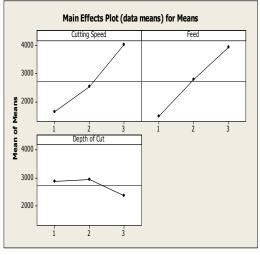
From Table 4, it is clear that feed is the most influencing factor followed by cutting speed and depth of cut for MRR. The optimum value for MRR is predicted from Fig 1, i.e. cutting speed of 938 rpm, feed of 0.1875 mm/rev and depth of cut of 0.3 mm.
