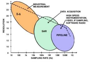
Fig 13: Graphical representation of ADC's.
