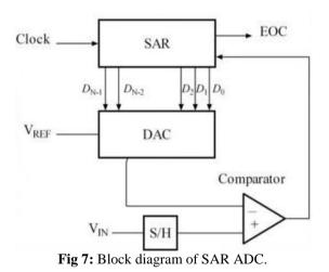
Advantages: For an N-bit ADC conversion time is equal to 'N' clock cycle. Hence the time required for conversion is small, Conversion time is constant and
