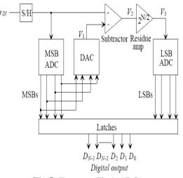
Fig 5: Two-step Flash ADC
