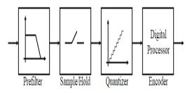
Fig 2:Working principle of an ADC.
