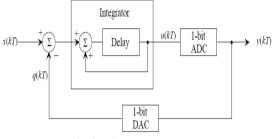
Fig 8: Sigma delta ADC.
