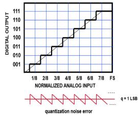
Fig 3: Quantization Process and quantization error.
