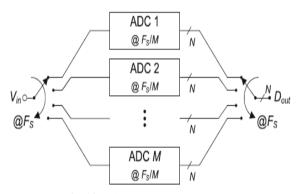
Fig 10: Time-Interleaved ADC.
