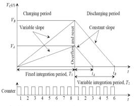
Fig 11: Characteristics of Dual-slope ADC.
