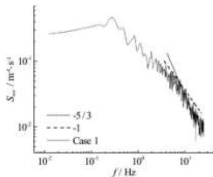
Fig.12 Powerspectral density of vertical velocity sampled at the top of the vegetation layer and a representative location ( $x/L_v=0.58$ )
