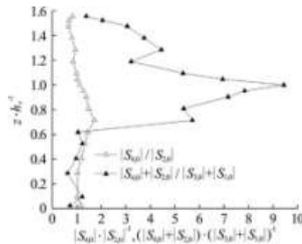
Fig.16 Ratio of contributions of various quadrant stomomen-tum transfer rate to representative cross-section in case 3
