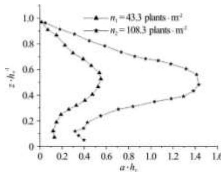
Fig.5 Variation of vegetation density along the vertical direction, where triangles indicate  $n=43.3$  plants/m<sup>2</sup>, and
