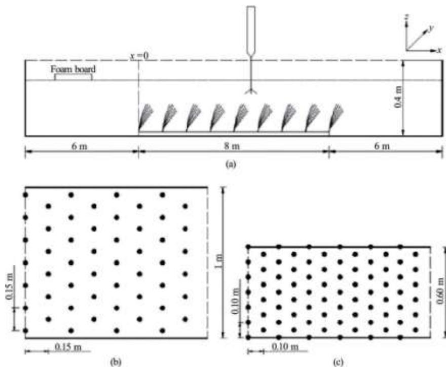
Fig.1 The experimental setup and vegetation placement in a rectangular channel (the layout is not to the scale) showing the longitudinal (a), plane (b) and cross-sectional (c) views. The  $z$  is the distance from the bottom of the channel, and  $h_v$  is
