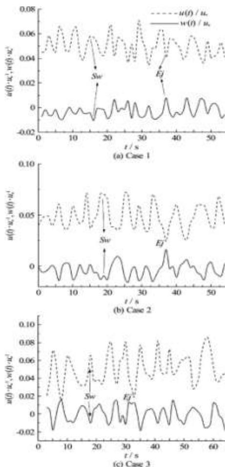
Fig. 11 Time series of longitudinal velocity and Reynolds stress versus time at a completely developed cross-section in
