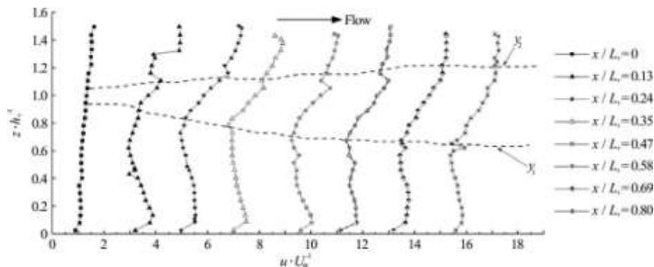
Fig.9 Development of the mean longitudinal velocity at various cross-sections in case 1. The thickness of the mixing layer is
