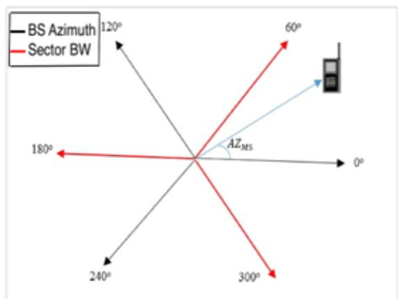
Fig. 1. Geometry for Gain Calculations
