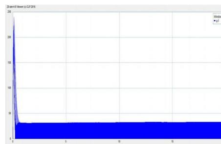
Fig 5 Valve seating velocity of the proposed system in 1000rpm.
