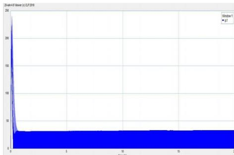
**Fig 7** Valve seating velocity of the proposed system in 3000rpm.
