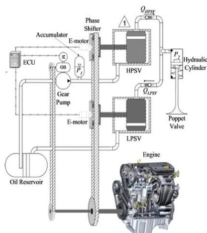
Fig 1 Schematic diagram of the variable valve actuation
