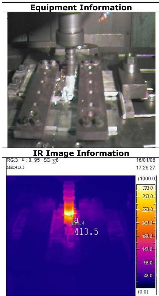
**Figure 4:** IR image for FSW of AA6082 T6 alloy with spindle speed 1000 rpm and welding speed 48mm/min,
