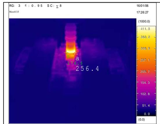
**Figure 5:** IR image at TMAZ region of FSW
