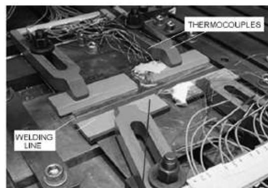
**Figure 1:** Thermocouples for measuring temperature during welding cycle
