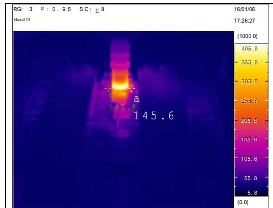
**Figure 6:** IR image at HAZ region of FSW
