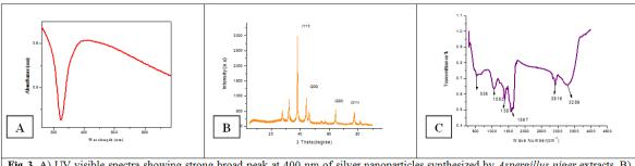
Fig 3. A) UV visible spectra showing strong broad peak at 400 nm of silver nanoparticles synthesized by *Aspergillus niger* extracts. B) X-ray crystallographic studies of silver nanoparticles. C) FT- IR spectra of silver nanoparticles.
