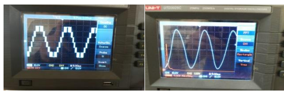
Fig. 17. The hardware output voltage using MSPWM: three level (A) without filter; (B) with filter and harmonics spectrum; five level (C) without filter; (D) with filter and harmonics spectrum; seven level (E) without filter; (F) with filter and harmonics spectrum
