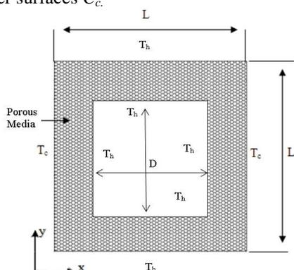
Fig. 1: Schematic of Porous Annulus
