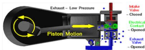
Fig. 2. 6. Final Position of Exhaust Stroke.
