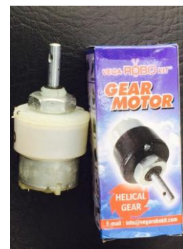
Fig.3 Geared DC Motor 1 (10 RPM)
