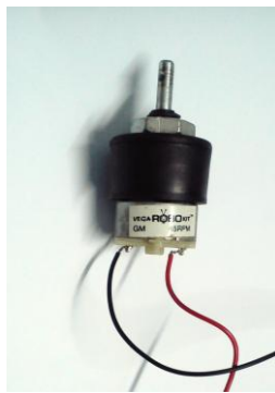
Fig.4 Geared DC Motor 2 (150 RPM)
