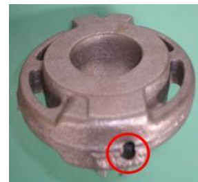
"Cold shut" defect on die cast part
