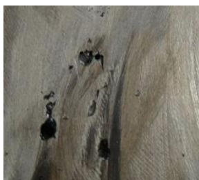
Sand inclusion defects
