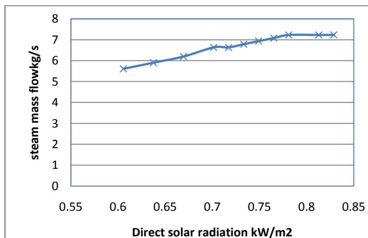
Fig. 7. Variation of the steam mass flow in the parabolic trough as a function of the solar radiation in the optimized configuration A.
