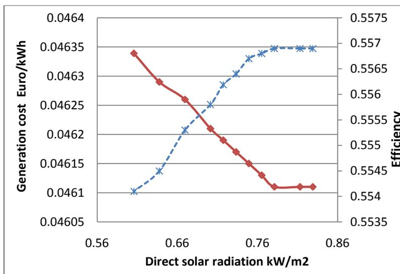
**Fig. 8.** Variation of the generation cost and efficiency of the ISCC as a function of the solar radiation in the optimized configuration A.
