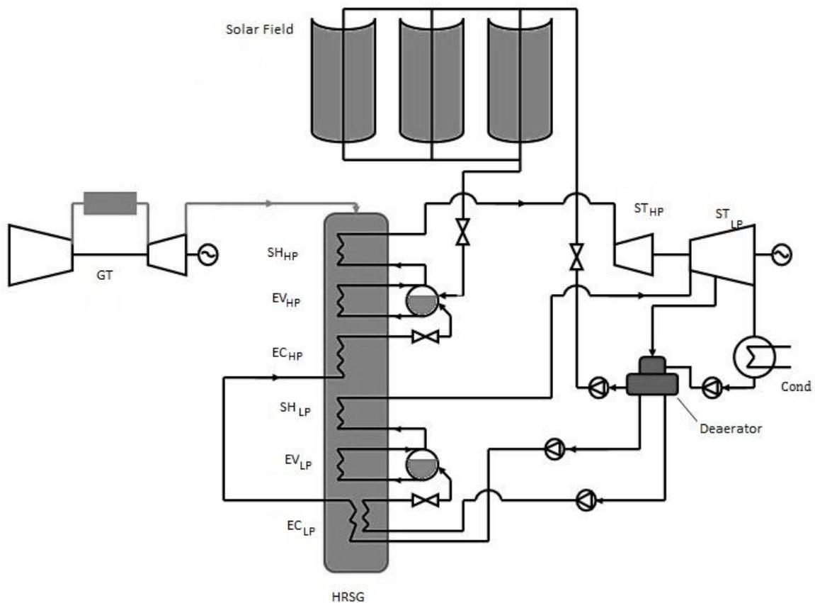
**Fig. 2.** Configuration A: CCPP with two pressure levels without reheater where the high pressure economizer is the solar field.
