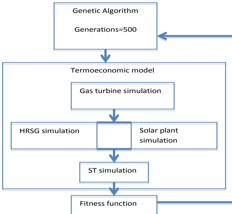
**Fig. 4.** Schema of the optimization program with all the simulation modules.
