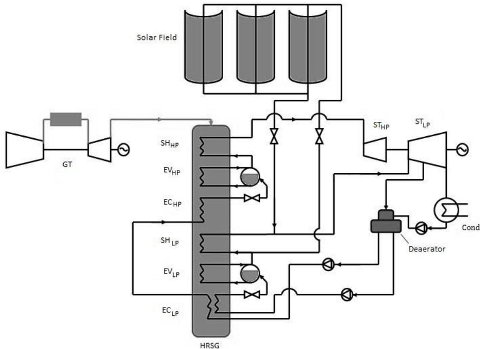
**Fig. 3.** Configuration B: CCPP with two pressure levels without reheater where the Low pressure superheater is the solar field.
