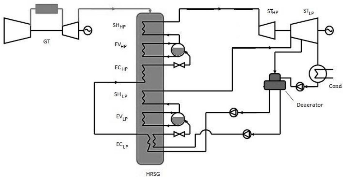
**Fig. 1.** CCPP with two pressure levels without reheater.
