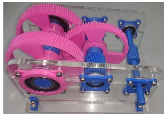
Fig. 11 Printed gears and shafts in the gear box
