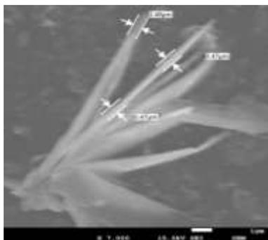
Fig.8. SEM image of as deposited CdZnTe<sub>2</sub> thin film at substrate temperature 300°C.
