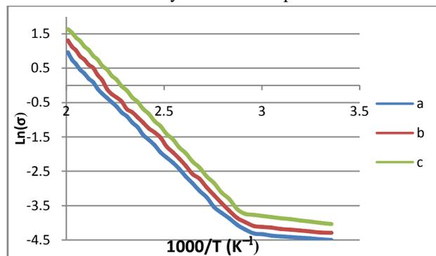
Fig.9 Arrhenius plots of as deposited CdZnTe<sub>2</sub> thin films at substrate temperatures a.250°C, b.275°C and c.300°C.
