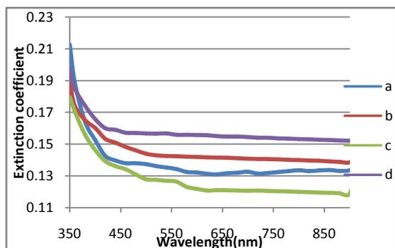
**Fig.5** Variation of extinction coefficient as a function of wavelength for CdZnTe<sub>2</sub> thin film at substrate temperatures. a.250°C, b.275°C, c.300°C, d.325°C.
