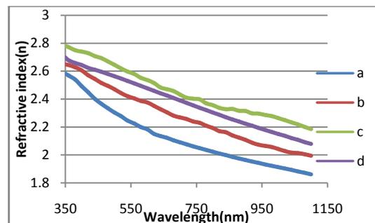
**Fig.4** Variation of refractive index as a function of wavelength for CdZnTe<sub>2</sub> thin films at Substrate temperatures a.250°C, b.275°C, c.300°C, d.325°C
