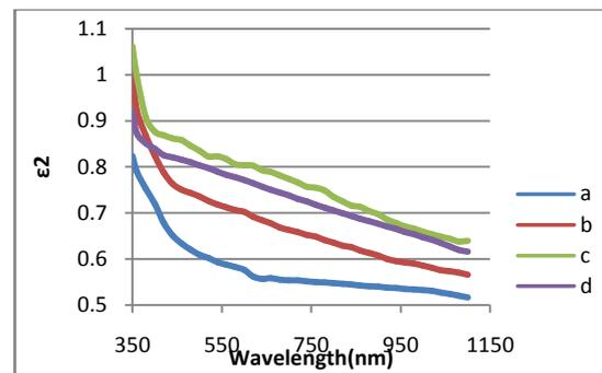
Fig.7 Variation of imaginary part of dielectric constant as a function of wavelength for CdZnTe<sub>2</sub> thin films at substrate temperatures a.250°C, b.275°C, c.300°C, d.325°C
