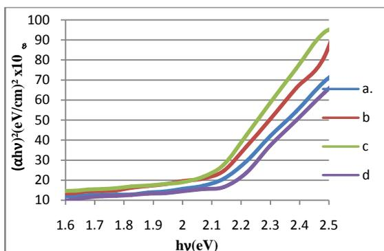
**Fig.2** Variation of  $(\alpha hv)^2$  as the function of photon energy for CdZnTe<sub>2</sub> thin films at Substrate temperatures a.250°C, b.275°C, c.300°C ,d.325°C
