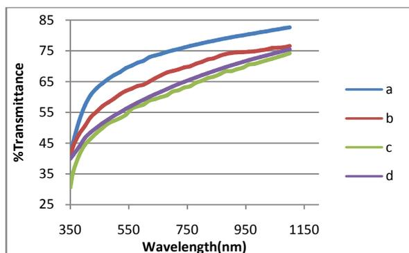
**Fig.1.** Transmission spectra of CdZnTe<sub>2</sub> thin films at Substrate temperatures a.250°C, b.275°C, c.300°C d.325°C.
