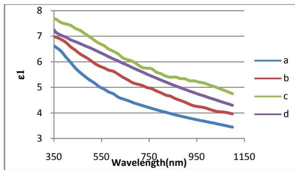
Fig.6 Variation of real part of dielectric constant as a function of wavelength for CdZnTe<sub>2</sub> thin films at substrate temperatures a.250°C, b.275°C, c.300°C, d.325°C
