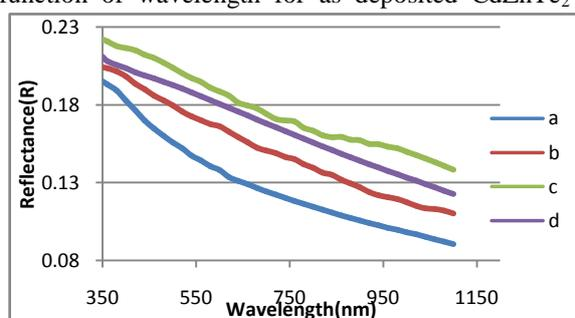
**Fig.3.** Reflectance spectra of CdZnTe<sub>2</sub> thin films at Substrate temperatures a.250°C, b.275°C, c.300°C, d.325°C
