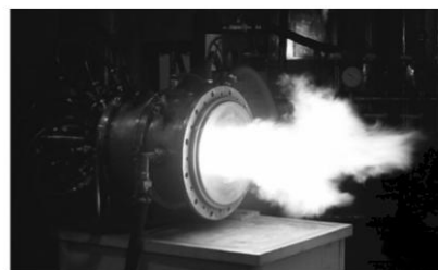
Figure 4. The photograph of the three-phase AC plasma torch of average power: power 30 kW, working gas – air [50].
