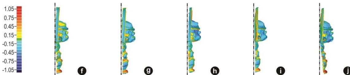
**Fig. 6** Dimensional analysis of wax injection to obtain the *Hombre Murciélago* models. Results of the comparison between the virtual reference model and the wax-injected pieces of Sample 1 (a,f), Sample 2 (b,g), Sample 3 (c,h), Sample 4 (d,i) and Sample 5 (e,j). Units expressed in mm.
