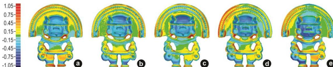
**Fig. 7** Dimensional analysis of the final pieces of the *Hombre Murciélago* obtained by investment casting. Results of the comparison between the virtual reference model and the final pieces of Sample 1 (a), Sample 2 (b), Sample 3 (c), Sample 4 (d) and Sample 5 (e). Units expressed in mm.
