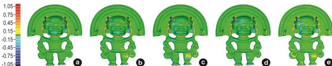
Fig. 4 Dimensional analysis of *Hombre Murciélago* models obtained by CNC machining. Results of the comparison between the virtual reference model and the CNC machining of Sample 1 (a), Sample 2 (b), Sample 3 (c), Sample 4 (d) and Sample 5 (e).
