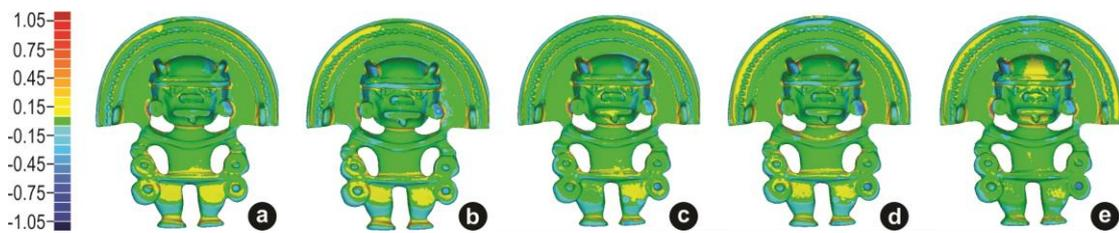
**Fig. 5** Dimensional analysis of *Hombre Murciélago* pilot pieces obtained by investment casting. Results of the comparison between the virtual reference model and the investment casting of Sample 1 (a), Sample 2 (b), Sample 3 (c), Sample 4 (d) and Sample 5 (e). Units expressed in mm.
