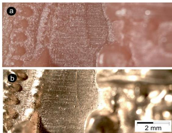
Fig. 3 Evaluation of results obtained with the pilot pieces for the surface finish: (a) the tool marks on the waxed models were reproduced in the metallic version (b) of the *Hombre Murciélago*.
