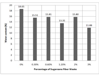
Fig.6.Water absorption percentage by percentage of sugarcane fiber waste
