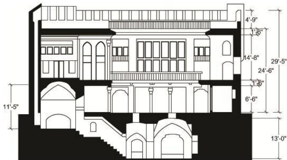
Figure 7: Section showing the relationship between the three levels of the house, the underground, ground level, and first floor.
