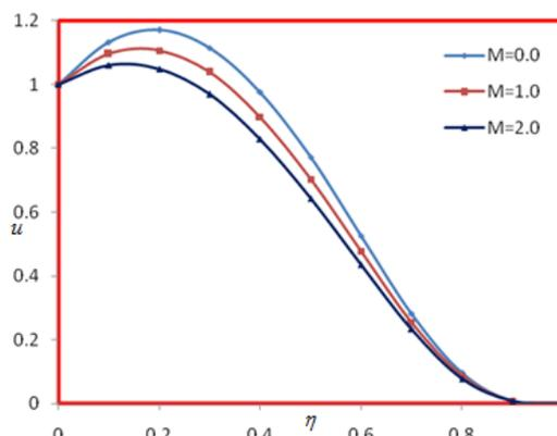
**Fig 2: Effect of Magnetic parameter  $M$  on velocity field  $u$**
