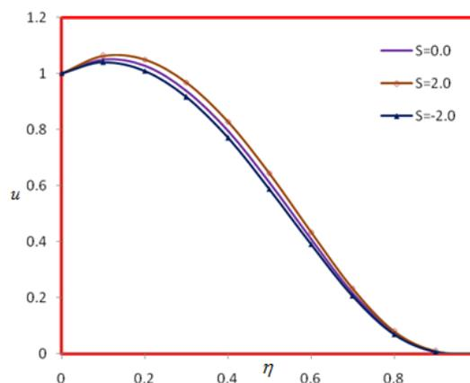
**Fig 1: Effect of heat source and sink on velocity field  $u$**
