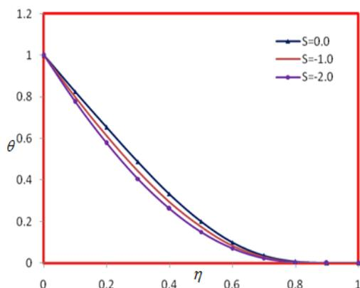
**Fig 4: Effect of heat Sink on temperature field**
