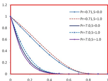
**Fig 5: Effect of Prandtl number in the presence of heat source/sink on temperature field**
