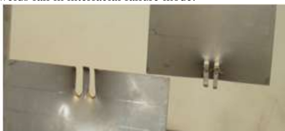
Fig.5 .Pull out failure mode
