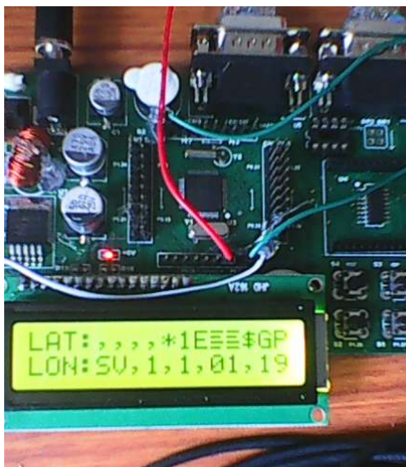
FIG-9: DISPLAY OF LONGITUDE AND LATITUDE WHEN FIRE ACCIDENT IS OCCURED
