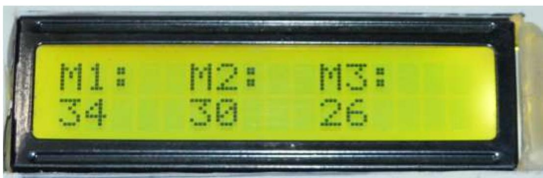
fig 4: displaying the values of three moisture sensors.
