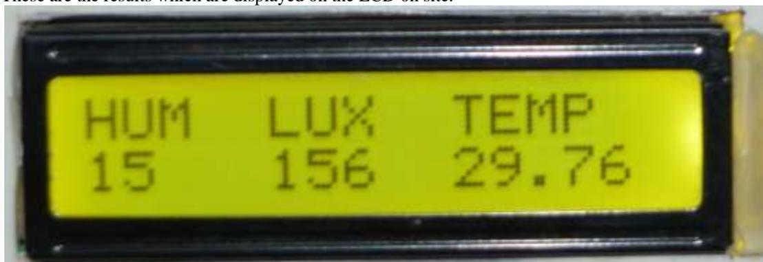
fig 3: displaying the values of humidity, light and temperature
