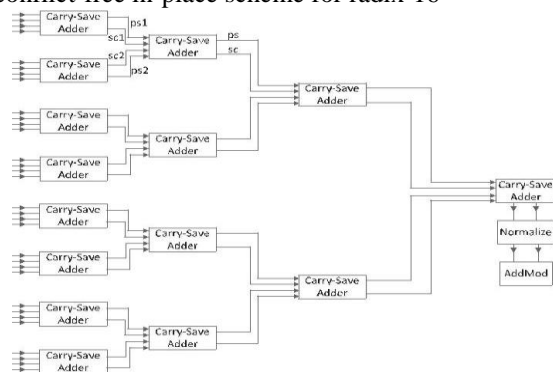
Fig. 3. Diagram of sum-16 unit.
