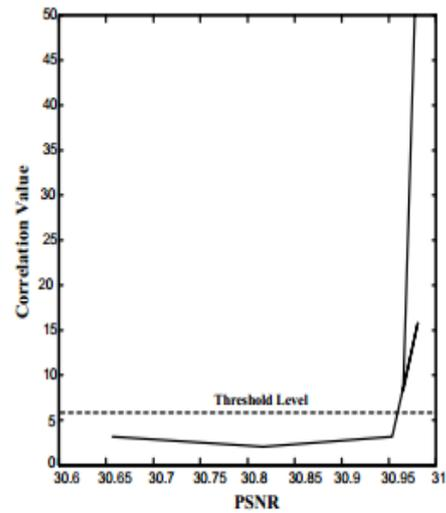
FIGURE IV. WATERMARK DETECTOR RESPONSE AGAINST DIFFERENT LEVELS OF ADDITIVE GAUSSIAN NOISE.
