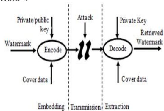
FIGURE I: GENERAL PROCESS OF IMAGE WATERMARKING
