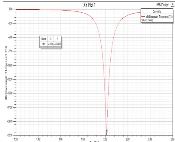
Fig(3) return loss with jean cotton as substrate
