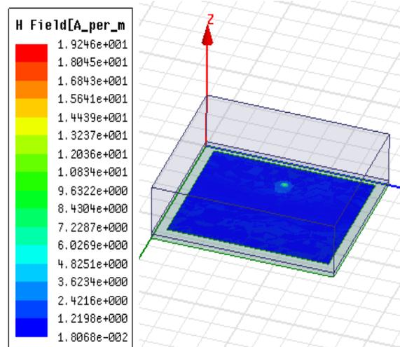
Fig (20) H-field with wash cotton as substrate
