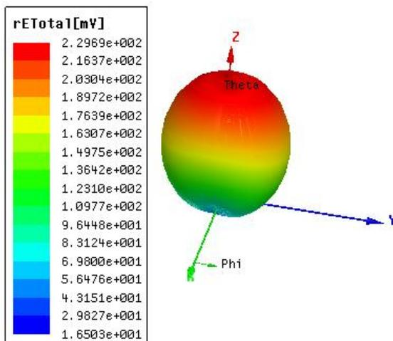
Fig (14) 3d radiation pattern with curtain cotton as substrate
