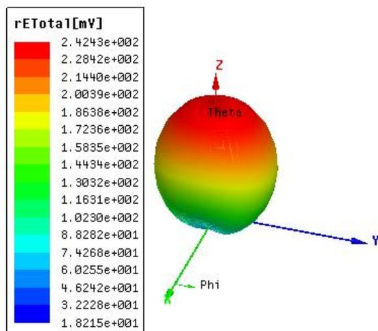
Fig (13) 3d radiation pattern with polycotton cotton as substrate
