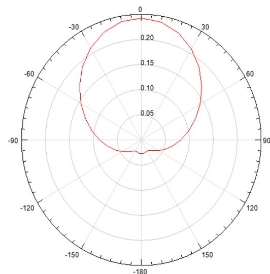
**Fig (9) 2d pattern with polycotton as substrate**
