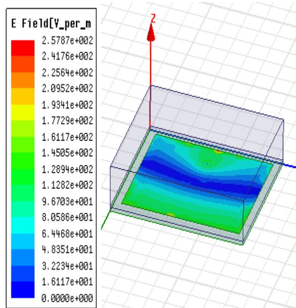
**Fig (16) E-Field pattern with wash cotton as substrate**
