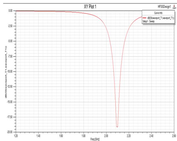
Fig (4) return loss with wash cotton as substrate
