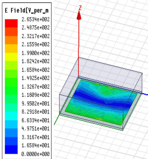
Fig (18) E-Field pattern with curtain cotton as substrate
