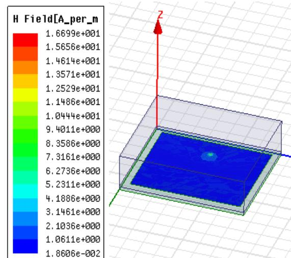
Fig (22) H-field pattern with curtain cotton as substrate
