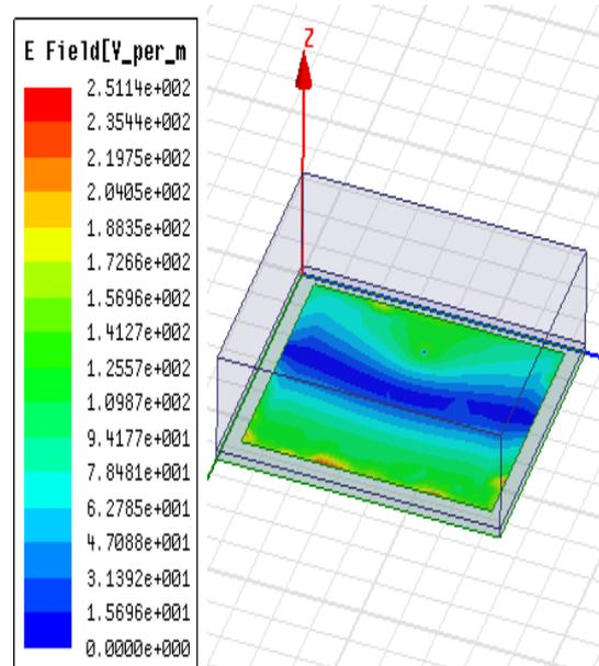
**Fig (17) E-Field pattern with polycotton cotton as substrate**
