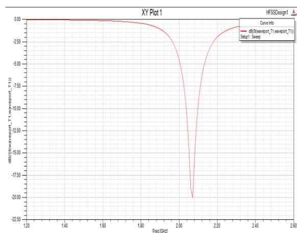
Fig (5) return loss with polycotton as substrate
