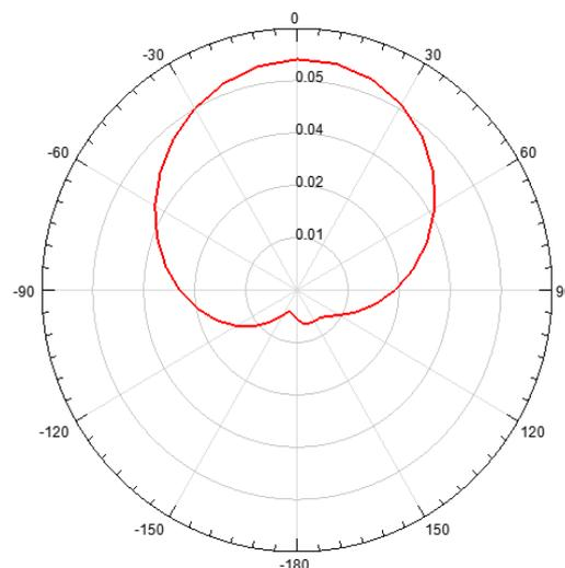
**Fig (8) 2d pattern with wash cotton as substrate**
