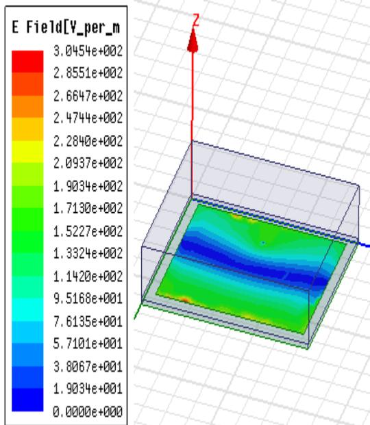
**Fig (15) E-Field pattern with jean cotton as substrate**
