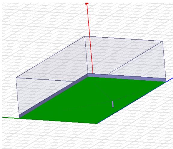
Fig (2) Patch Antenna with coaxial feed
