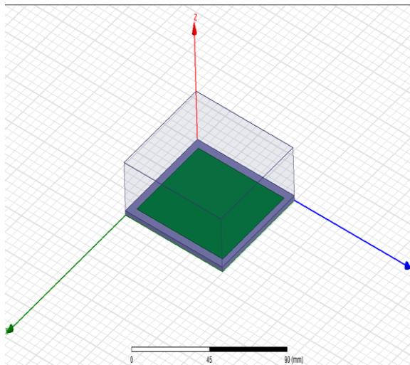
Fig (1) Microstrip Rectangular Patch Antenna
