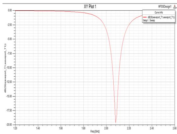
**Fig (6) return loss with curtain cotton as substrate**
