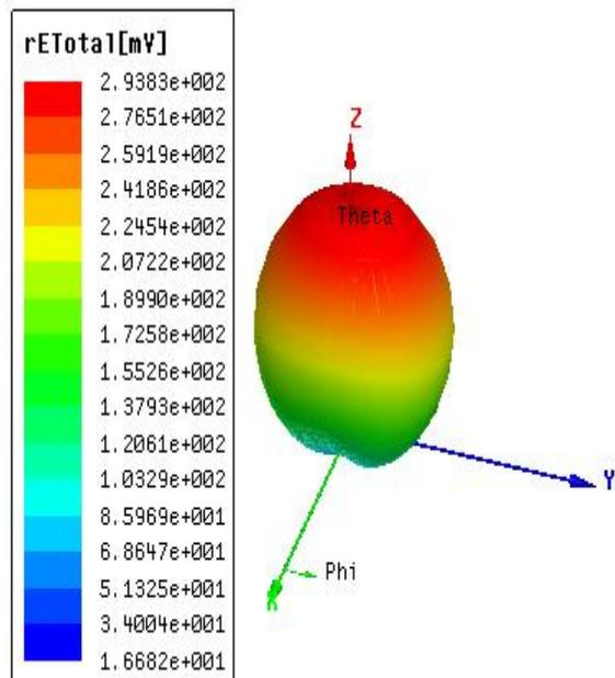
Fig (11) 3d radiation pattern with jean cotton as substrate
