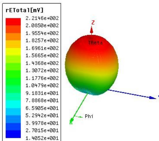
Fig (12) 3d radiation pattern with wash cotton as substrate
