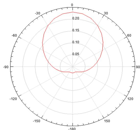
**Fig (10) 2d pattern with curtain cotton as substrate**
