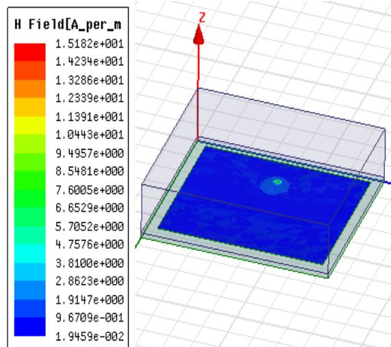
Fig(21).H-field pattern with polycotton as substrate
