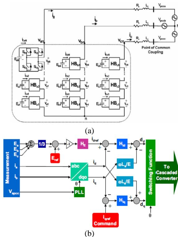
Fig.3.Proposed STATCOM and its controller.(a) Generalized CMC-based Y-connected STATCOM schematic. (b) Internal control strategy of CMC-based STATCOM.
