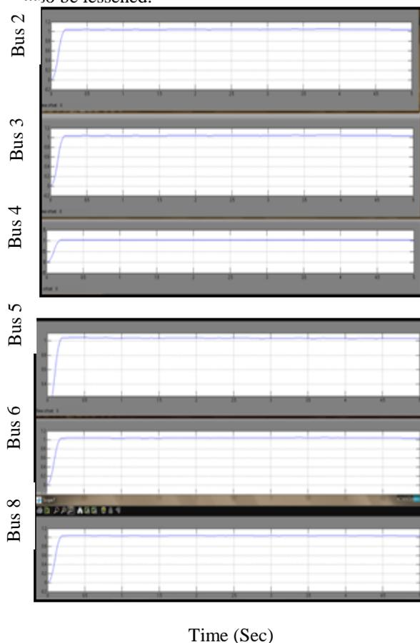
Fig.5. Simulation Results of Bus Voltages with STATCOM
