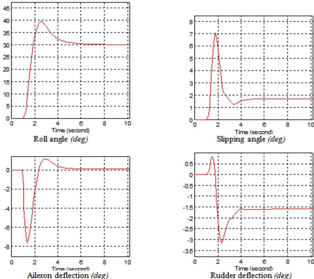
**Fig.1.** ‘Simulink’ results of the transient process after setting a desired roll angle in the astatic autopilot
