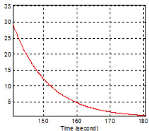
Fig.5. Change of flight altitude  $H(m)$  in the last seconds of automatic landing
