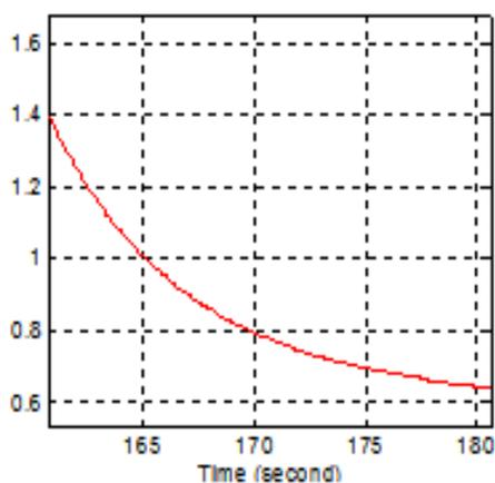
Fig.4. Decreasing of the lateral deviation  $\Delta Z(m)$  before landing on the runway under side-wind from the left of the airplane with 2 m/s. The landing is programmed with correction to the course.
