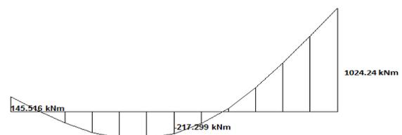
Fig 10. Beam with max bending moment
