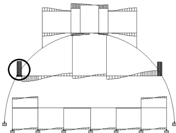
Fig 12. Shear force diagram.
