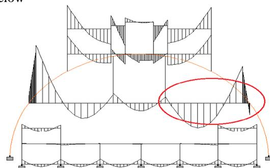
Fig 9. Bending moment diagram.
