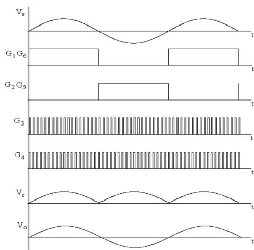
Fig. 4. Related control signals of the power
