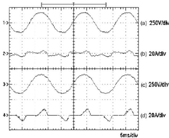
Fig. 11. Experimental results of the proposed AVR under a utility voltage of 121 V and nonlinear load. (a) Utility voltage. (b) Utility current. (c) Load voltage. (d) Load current.
