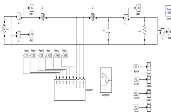
Fig 9: shows the simulink of proposed AVR. It includes source, subsystem1, subsystem2, and load.
