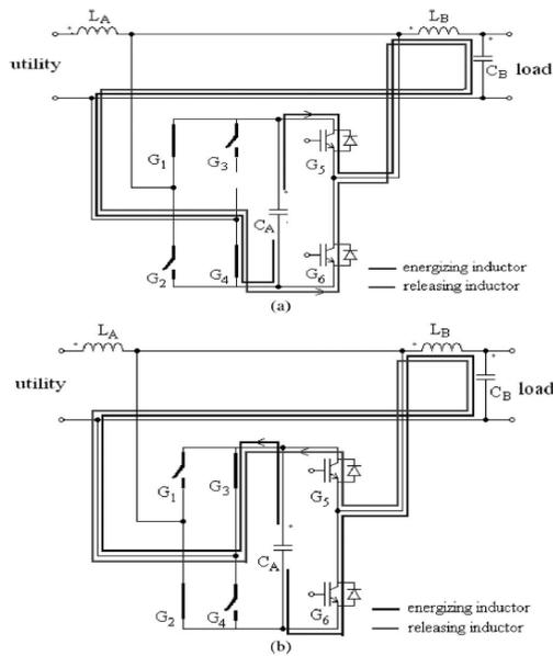
Fig. 5. Operating circuit of the proposed AVR under the ac buck mode (a) Positive half-cycle. (b) Negative half-cycle.
