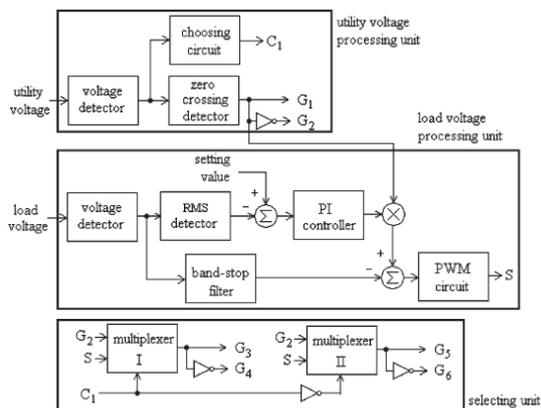
Fig. 7. Control block of the proposed three-arm power converter.
