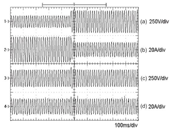
Fig14: Experimental results of the proposed AVR upon changing the utility voltage abruptly from 77 to 143 V. (a) Utility voltage. (b) Utility current. (c) Load voltage. (d) Load current.
