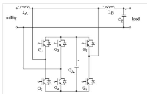
Fig 2: Circuit configuration of the proposed three-arm AVR.
