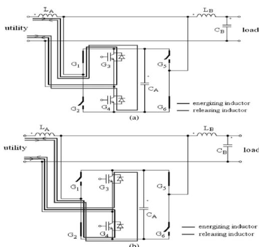
Fig. 3. Operating circuit of the proposed AVR under the ac boost mode. (a) Positive half-cycle. (b) Negative half-cycle.
