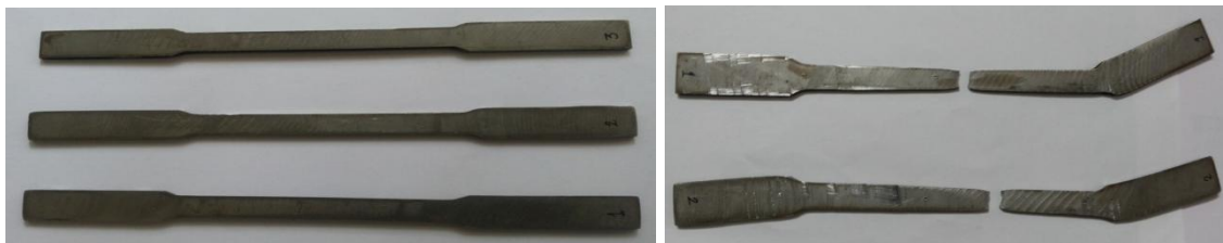
(b) Specimen casted from SS 304 having thickness of 3 mm (c) Failure pattern of SS Specimen
