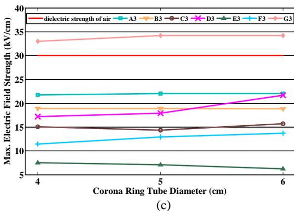
Figure 7. Regional  $E_{max}$  versus corona ring tube diameter. (H=20cm, D=50cm), (a) first insulator, (b) second insulator, (c) third insulator
