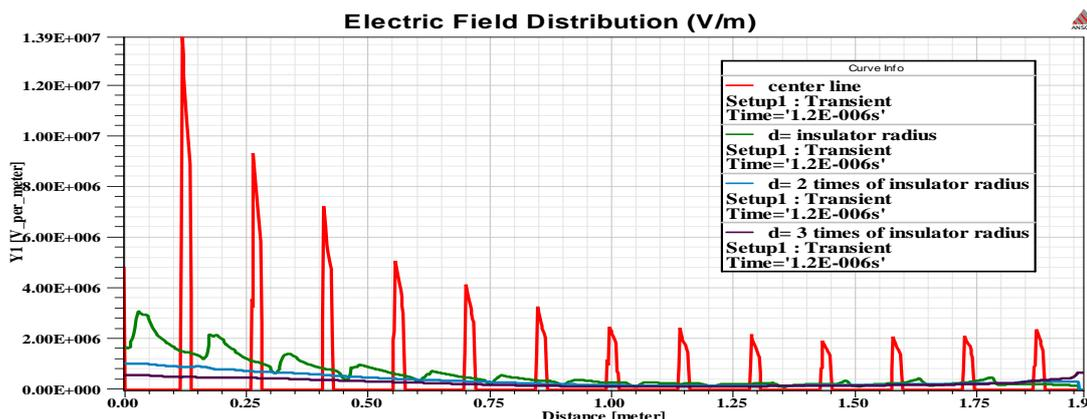
Figure 3. Electric field strength along lines parallel to the insulator axis (at different distance)
