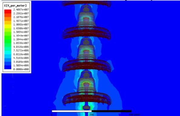
Figure 4. Electrical field contours around three line-side insulator units
