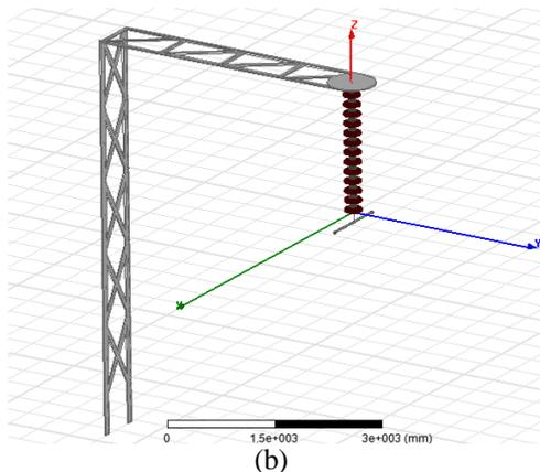
Figure1. (a) Basic dimensions of cap and pin type porcelain insulator unit, (b) Simplified 3-dimensional simulation model of tower
