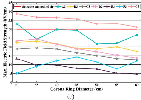
Figure 6. Regional E<sub>max</sub> versus corona ring diameter. (H=20cm, R=4cm), (a) first insulator, (b) second insulator, (c) third insulator
