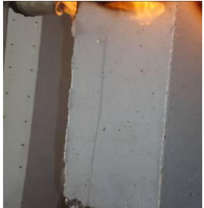
Fig. 18-Runoff water from SCC column specimen.
