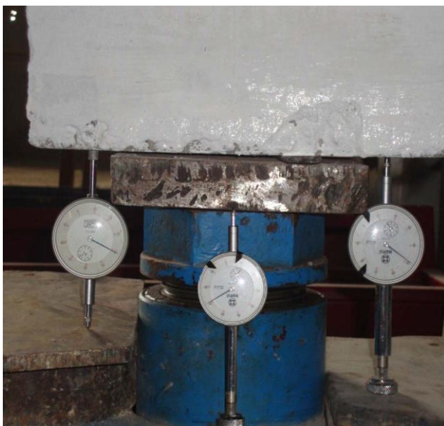
Fig. 6-The testing measurement of axial deformation.
