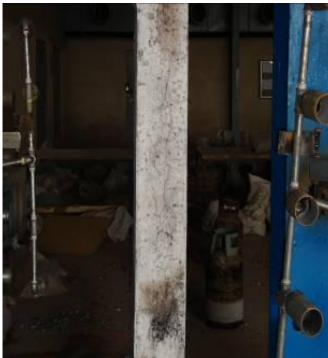
Fig. 15-Formation of longitudinal cracks due to exposure to fire 752°F (400°C) and concentric loading. Note: tC = (tF - 32)/1.8
