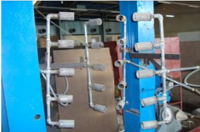
Fig. 4-The network methane burners.
