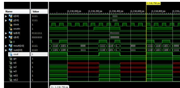
Fig 5 .Error output due to fault in the circuit
