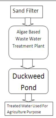
Figure-1. Model of the proposed wastewater treatment for aquaculture purpose.
