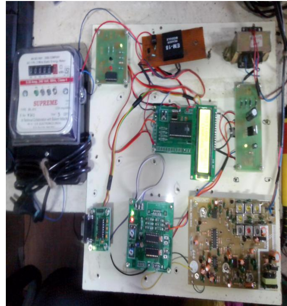
Figure2: Power Data Transmitter
