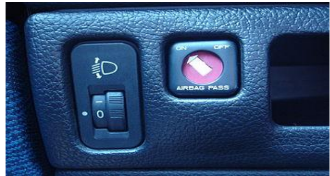
Figure 4: ON/OFF switch of air bag system
