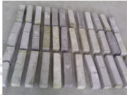
Fig No.3 Part of the Beam specimens after ultimate failure
