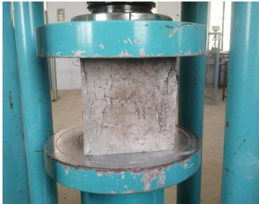
Fig No.1 Crack pattern at ultimate failure load of Cube specimen
