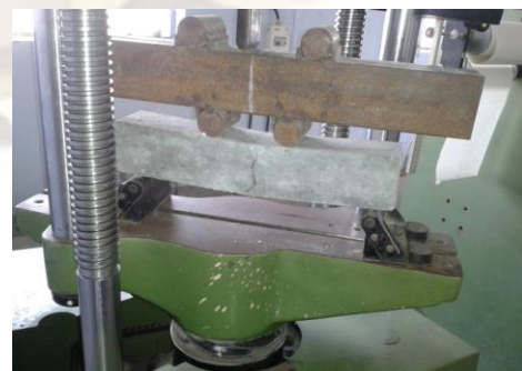
Fig No.2 Flexural strength setup
