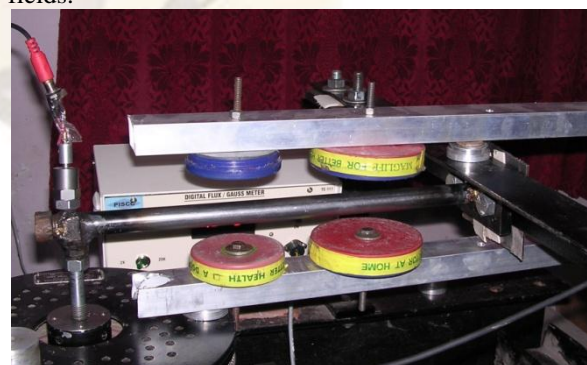
Figure 3 Experimental setup for MR sandwich beam with applied magnetic field
