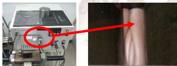
Figure 5 (a) Brabender Mixer (b) Compounding process of Copper, ABS and surfactant Material
