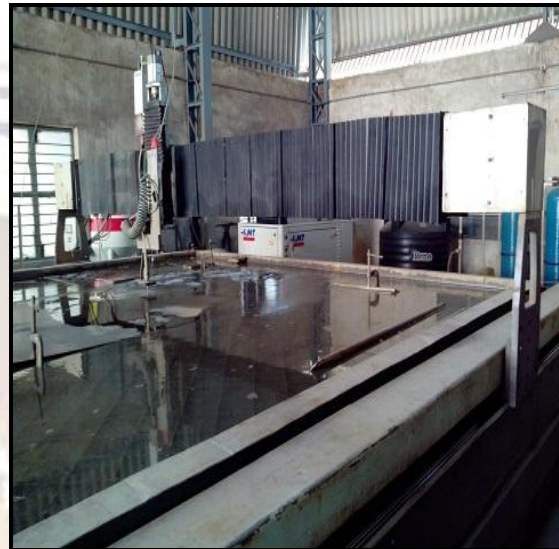
Fig: 2 - Setup of AWJM with Cutting table
