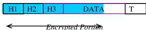
Figure 5. Network Layer Encryption. In this case, data and more headers are encrypted. Here H1 , H2 and H3 are headers and T is trailer.
