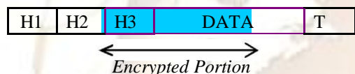
Figure 7. Application Layer Encryption. In this case, only data portion is encrypted. Here H1 , H2 and H3 are headers and T is trailer.
