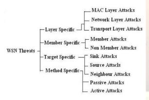
Fig 1.1: Types of Threats in Wireless Sensor Network
