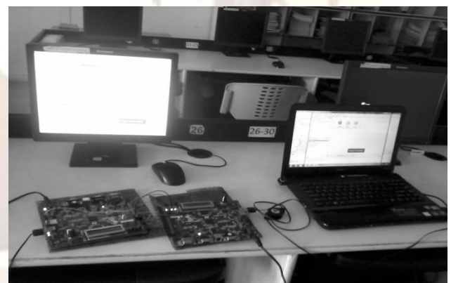
Figure 3. FPGA based virtual motor experimental setup
