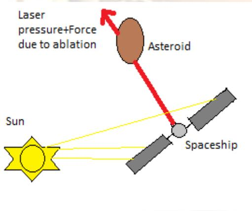
Figure 7. A Diagram showing Laser ablation and Laser pressure forces acting in the same direction
