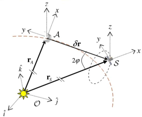
Figure 6. Definition of relative reference frames  $\mathcal{A}$  is centered on the asteroid  $\mathcal{S}$  is centered on the spacecraft.
