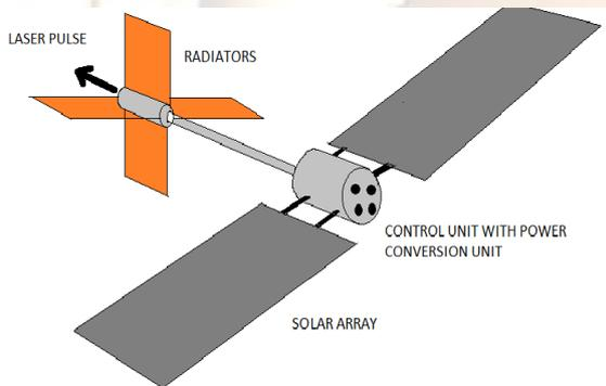
Figure 1. A model spacecraft with solar laser system
