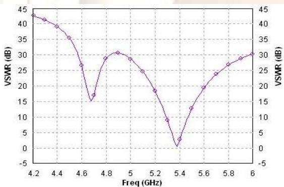
Figure.3. VSWR vs. Frequency plot for Table 1, VSWR is 1.2 at this location (3, 1)
