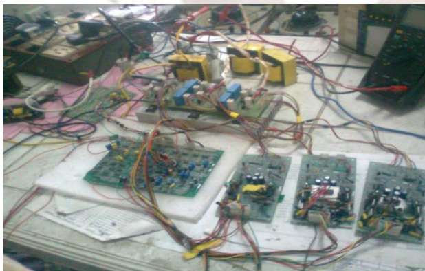
Figure 8: Experimental setup of the rectifier circuit
